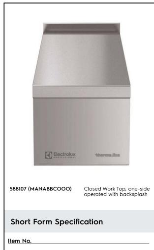
Closed work top, 300 mm wide, constructed according to DIN 18860\_2 with 20 mm drop nose top. Internal frame for heavy duty sturdiness in stainless steel. 2 mm top in 1.4301 (AISI 304). Flat surface construction, easily cleanable. THERMODUL connection system enables seamless worktop when units are connected and avoids soil penetrating.
